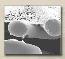
Ultra-Web nanofiber media has submicron diameters and small interfiber spaces, resulting in the contaminant being captured on the surface of the media, greatly improving filtration efficiency and making effective pulse cleaning possible.
