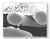
Ultra-Web nanofiber media has submicron diameters and small interfiber spaces, resulting in the contaminant being captured on the surface of the media, greatly improving filtration efficiency and making effective pulse cleaning possible
